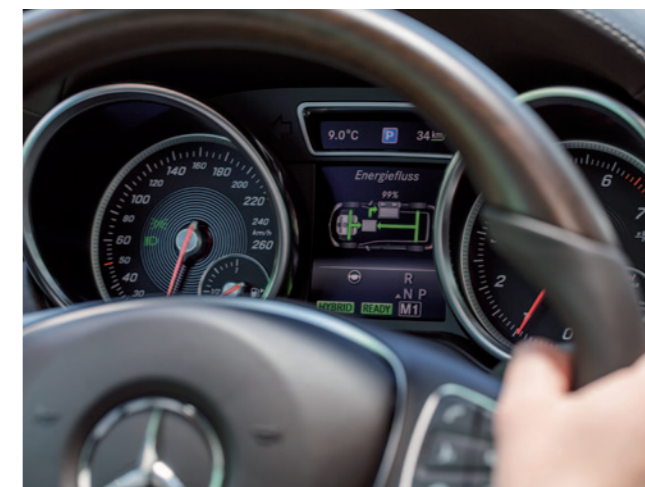
When the driver enters a destination in the navigation system, the intelligent operating strategy selects the optimum combination of electric motor and combustion engine for providing drive power along the specific route.
